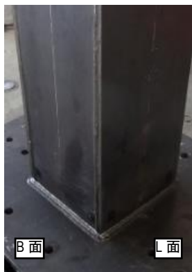
(i) B-L 面柱脚部詳細
